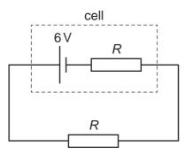
Power *P* is dissipated by the external resistor.
